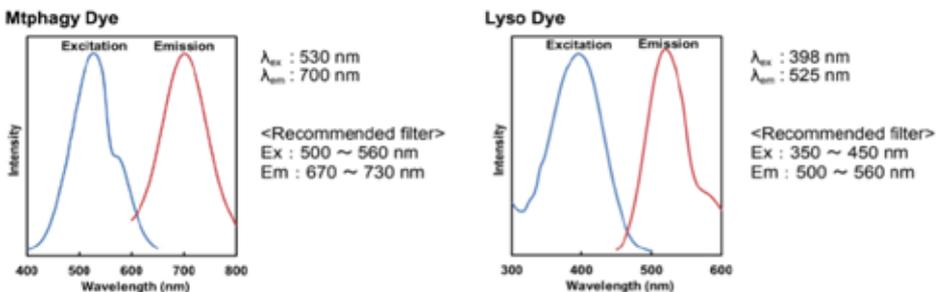
Figure 3. Excitation and emission spectra of Mtphagy Dye and Lyso Dye.
